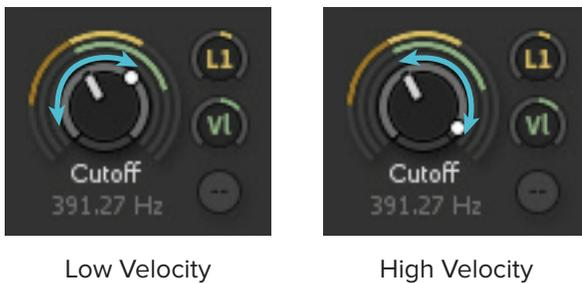
The figure above illustrates how the LFO's modulation shifts as it is added to the velocity of a MIDI note. The figure on the left is a lower-velocity note and the figure on the right is a higher-velocity note.
