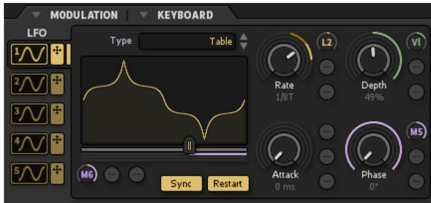
When a **Low Frequency Oscillator (LFO)** is applied to a Modulation Knob or Slider, that LFO will cause the parameter value to oscillate in a bipolar fashion around the center point of the knob. This pattern is decided by the shape of the LFO wavetable chosen in the LFO Type menu. By default the LFOs will start with a table of sine waves. If you drag the waveform display or Shape Slider located below it, you will interpolate between the shapes in the LFO wavetable.
